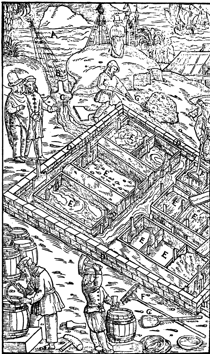
Figure 3. Making salt in ancient times: (A) sea; (B) pool; (C) gate; (D) trenches; (E) salt basins; (F) rake.
