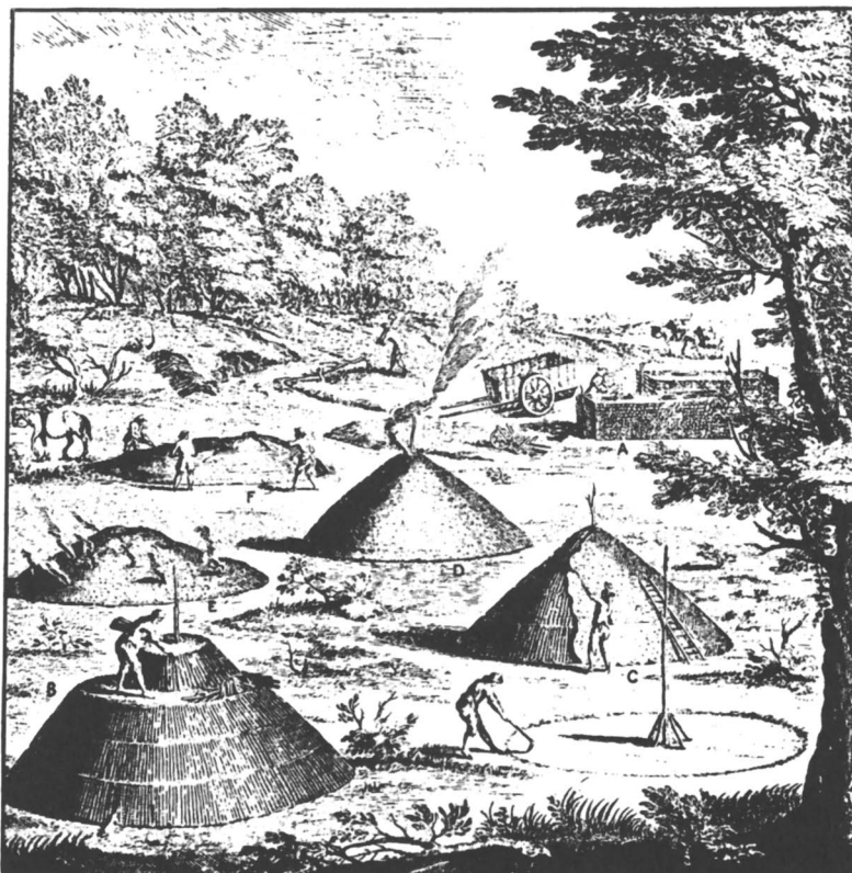
Figure 1. Charcoal burning: (A) wood-stack; (B) preparing the heap of wood; (C) covering it; (D) a freshly lit heap; (E) a nearly burnt-out heap; (F) uncovering a carbonized heap (5).
