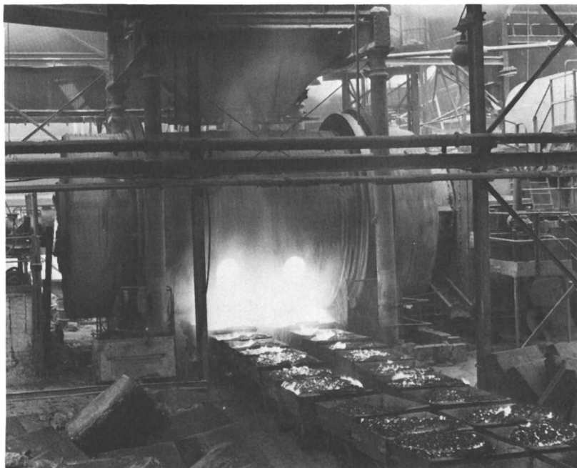
Figure 9. Late Victorian “black-ash revolver,” a revolving furnace used in the second stage of the Le Blanc process (18)
